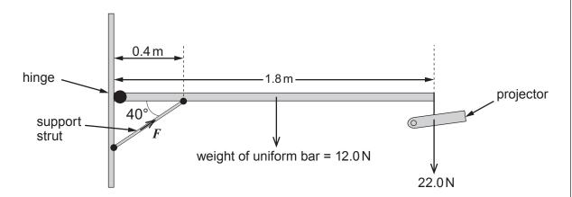
(i) By taking moments about the hinge, show that the force, F, exerted by the support strut on the uniform bar is approximately 200 N. [3]
