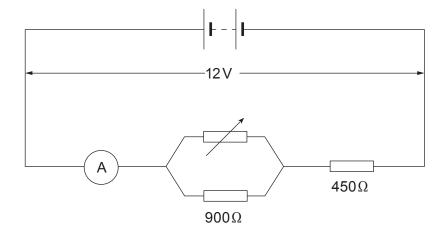
The variable resistor is adjusted so that the ammeter reads 0.01 A.
